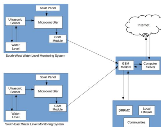
Figure 2. System Architecture
