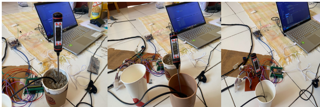
Figure 21. DS18B20 Readings in Comparison with Digital Thermometer
